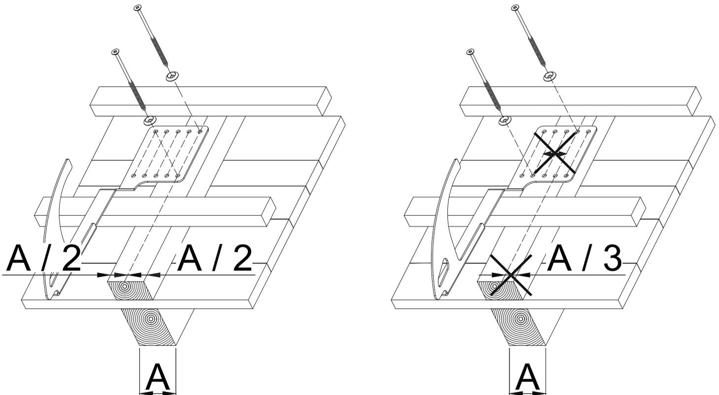
Align the roof hook in such a way that the 2 pcs. of supplied fixing screws, including form discs, can be fastened in the middle of the rafter. Depending on the height of the tile, height differences can be compensated by bending the Z-edge.
