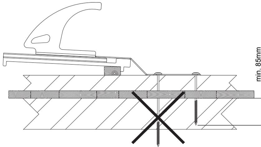
Fastening must be done with the original, supplied wooden construction screws, because only these achieve the required strength on the mounting surface.
