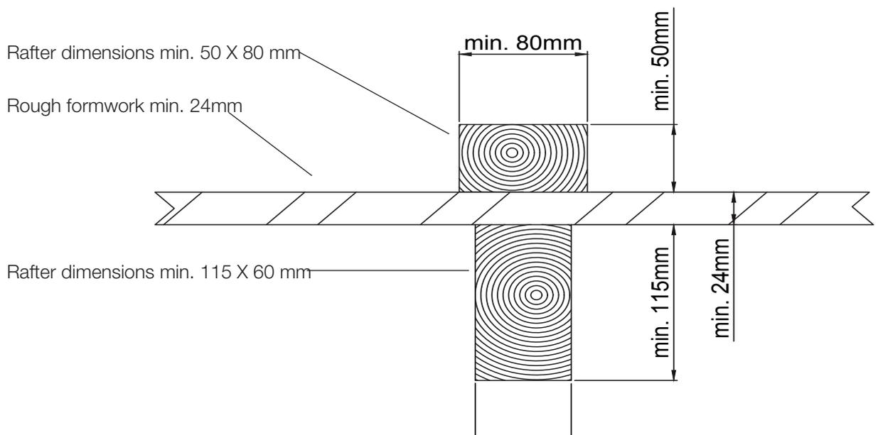
There must be a static load-bearing substructure. If in doubt, a structural engineer should be consulted.
